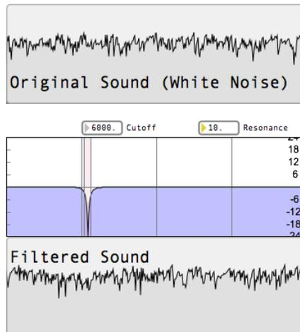
FIGURE 13. Band Pass Filter with high Resonance.
