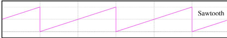
FIGURE 2. Sawtooth Wave [1].
