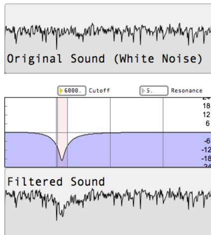
FIGURE 15. Peak Notch Filter with high Resonance.
