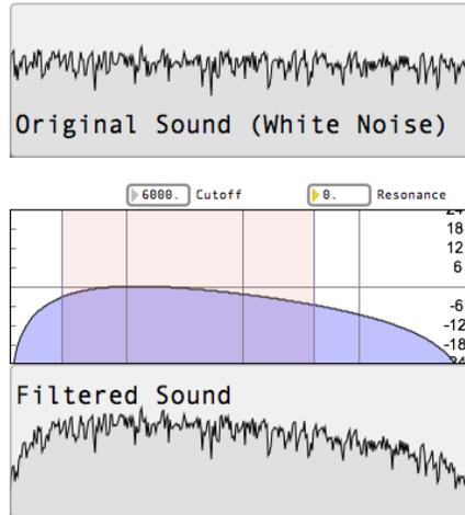
FIGURE 10. Band Pass Filter with low Resonance.
