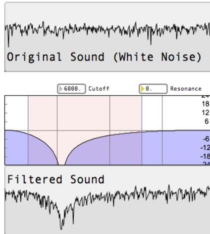
FIGURE 12. Band Stop Filter with low Resonance.
