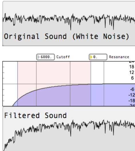
FIGURE 8. High Pass Filter with low Resonance.
