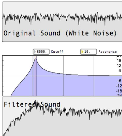
FIGURE 9. High Pass Filter with high Resonance.
