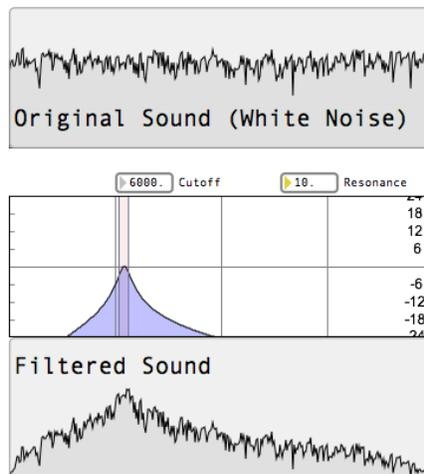
FIGURE 11. Band Pass Filter with high Resonance.
