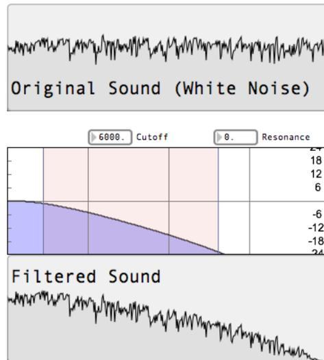
FIGURE 6. Low Pass Filter with low Resonance.
