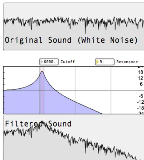
FIGURE 7. Low Pass Filter with high Resonance.
