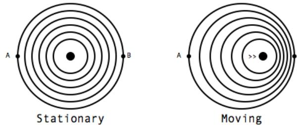
FIGURE 4. “Doppler Shift Effect” - As source is moving towards point B, the frequency is stretched (i.e. becomes longer - lower pitch) behind, and contracted (i.e. becomes shorter - higher pitch).
