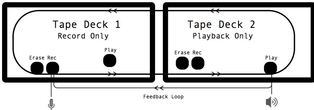
FIGURE 3. “Time-Lag Accumulator.” i.e. [Tape] Delay with feedback (Output of ‘play head’ is “fed back” into delay loop).
