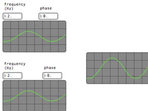
FIGURE 8. Two identical, **in phase**, sine waves are added together to create higher peaks and lower troughs.
