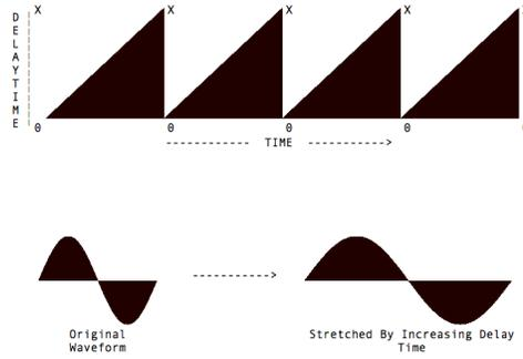
FIGURE 5. Increasing delay time at a constant rate to lower pitch of sound.
