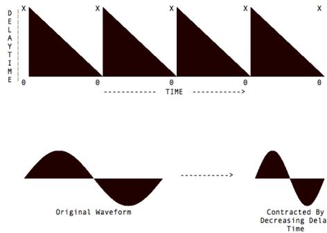
FIGURE 6. Decreasing delay time at a constant rate to higher pitch of sound.
