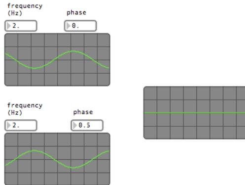
FIGURE 7. Two identical, **out of phase**, sine waves cancel each other out creating silence (this is essentially how noise cancelling headphones work).
