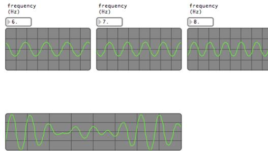
FIGURE 9. Multiple different sine waves added together produce a more complex sound. This is the basis of all the sounds we hear, a complex combination of sine waves.
