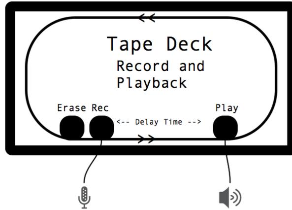
FIGURE 1. Basic [Tape] Delay (Distance between 'record head' and 'play head' determines 'Delay Time').
