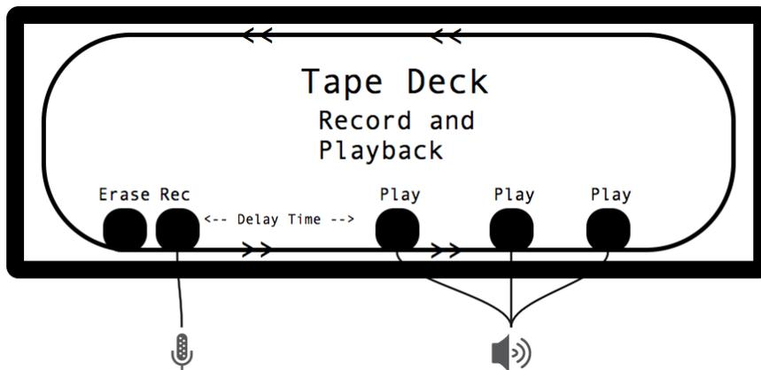
FIGURE 2. Multitap [Tape] Delay (Multiple 'play heads' means multiple repetitions of sound).
